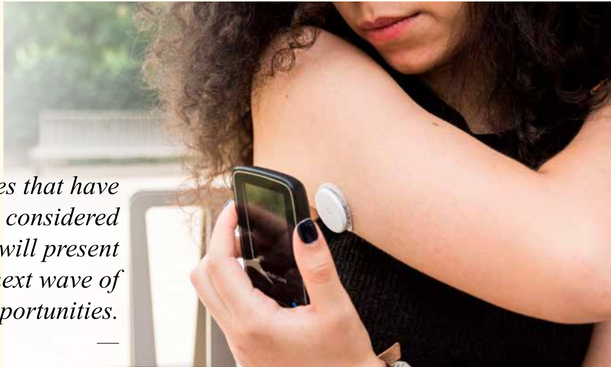
Glucose sensor and Freestyle Libre scanner which can just be flashed at the sensor on the back of arm to instantly measure blood sugar levels. © Universal Images Group/Getty Images.
